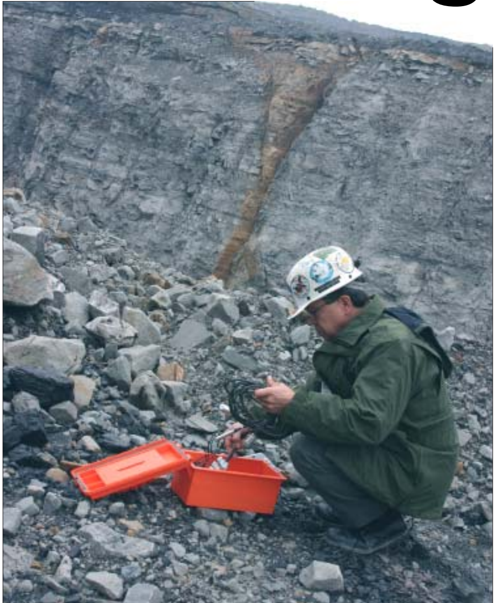
Darrell O'Brien is an inspector supervisor in the Office of Explosives and Blasting within the DEP. He sets out a seismograph at the Samples Mine in Eskdale.
