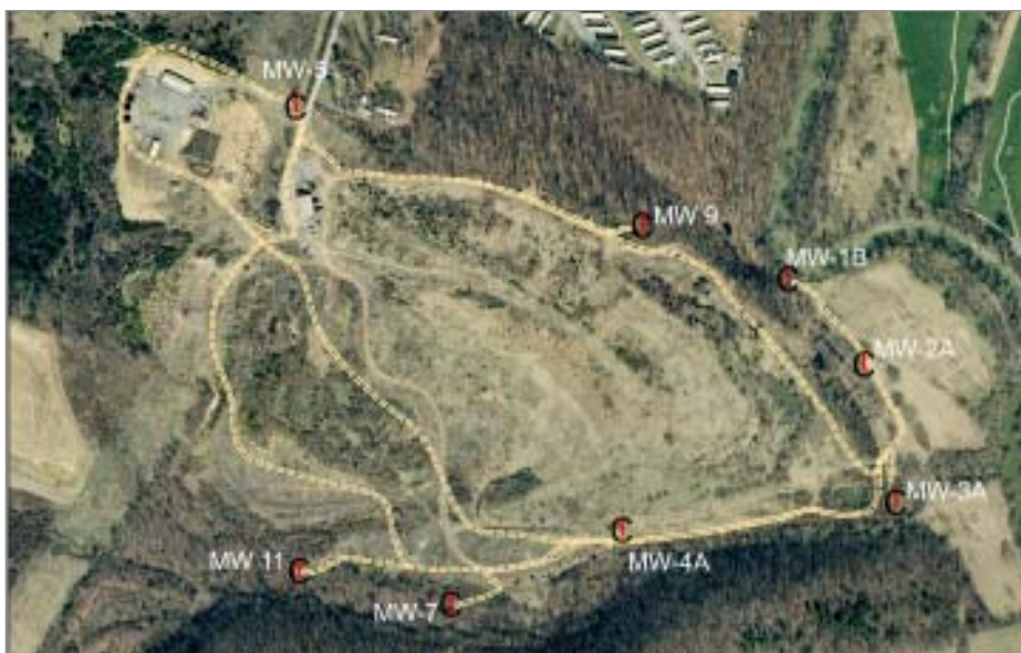
This aerial photo of the landfill shows the location of its monitoring wells.
